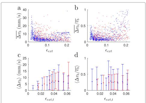
**Fig. 4 a** Band velocity fluctuations as a function of strain for experiments (red) and simulations (blue). **b** Same as a but for relative velocity fluctuations. **c** The average velocity fluctuations as a function of strain rate for experiments (red) and simulations (blue). **d** Same as c but for average relative velocity fluctuations
