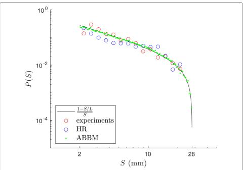
**Fig. 5** The distribution of band propagation distances (or avalanche sizes) in the experiments (red) in the Hähner–Rizzi model simulations (blue), and the ABBM model simulations (green). The black line represents the expected form of the distribution  $P(S) = A(1-\frac{S}{L})/S$  where  $A = \left(\frac{S_0}{L} + \ln \frac{L}{L_0} - 1\right)^{-1}$  and  $S_0 = 2$  mm
