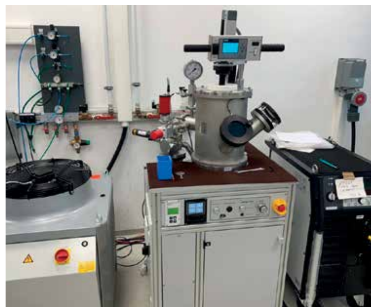
Figure: Arc melting device at NOMATEN. It will allow melting samples of up to approx. 200 g at temperatures up to 3500°C
