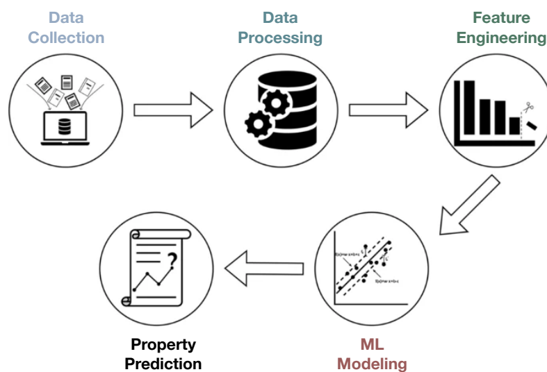
Figure 2. Main steps towards property predictions through the use of ML frameworks, driven by feature engineering in materials science. For mechanical deformation, multiscale microscopy and testing experimental data, as well as multiscale modeling data are used as input, that may exceed 1PB. From there, a key step involves data processing and reduction approaches [45,46], that may allow the derivation of meaningful features that capture key physical mechanisms. As soon as features are consistently defined, property prediction and machine learning models are built. Currently, the biggest challenge is focused on feature engineering and data management. Redrawn based on Ref. [47].
