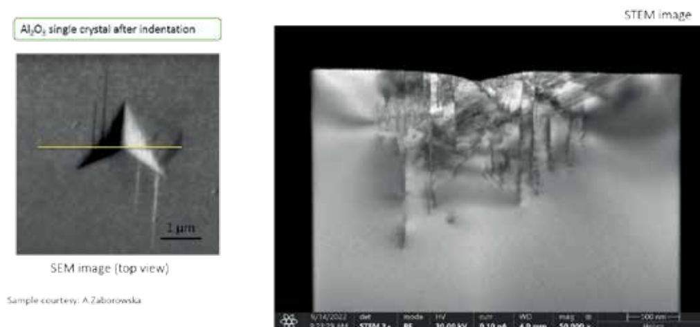
Fig. 4. S-TEM (scanning electron microscopy in transmission mode) image of crystalline \text{Al}_2\text{O}_3 after nanoindentation test. The site-specific FIB lift-out preparation of the thin foil allowed to obtain the transparent film of the sample at defined line of the cross section. The position of the line of cut was established by SEM imaging of the sample surface and nanoindentation mark (pile-ups and slip traces related to the material deformation are visible in both images).
