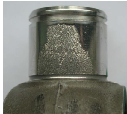
Macroscopic observation of the drive shaft cross after dynamic testing according with manufacturer quality control system – visible pitting effects
