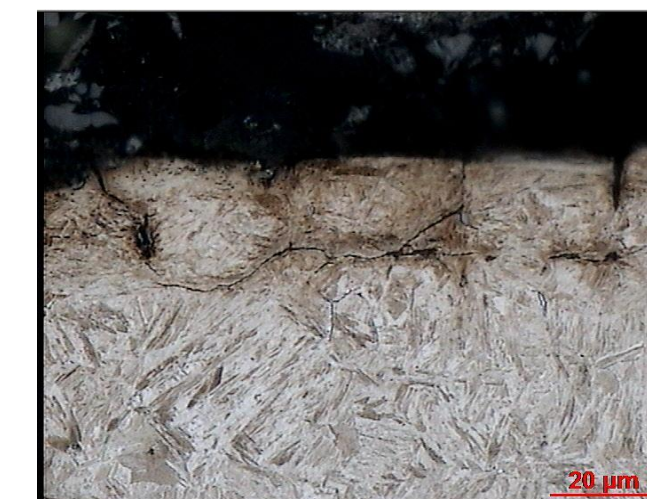
Microstructure analysis of low-alloy steel – surface cracking effects after induction hardening
