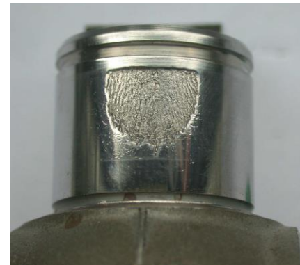
Macroscopic observation of the drive shaft cross after dynamic testing according with manufacturer quality control system – visible pitting effects
