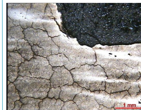
Macroscopic observation – visible blue brittleness > ca. 350 °C
