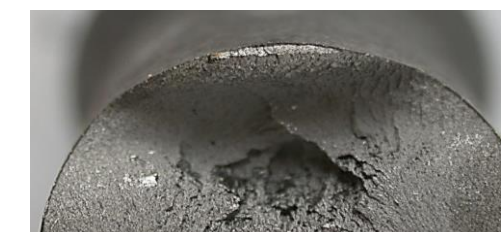
Microstructure analysis of low-alloy steel – surface cracking effects after induction hardening
