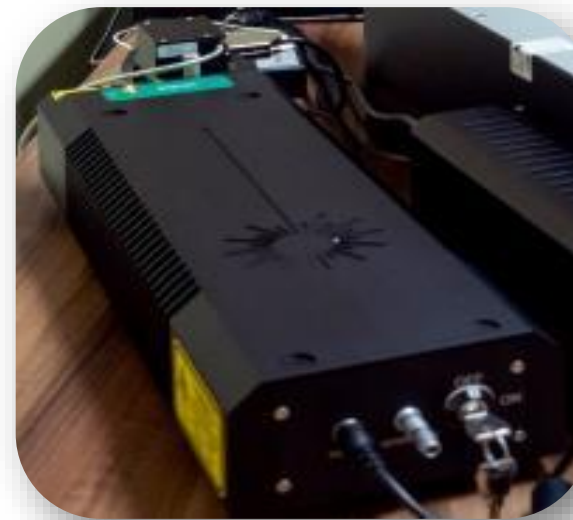
Ultra-high throughput spectrometer (UHTS), for high speed and high resolution Raman imaging.
