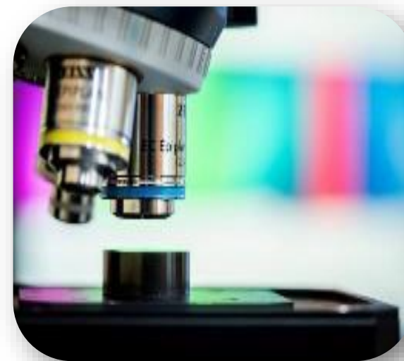
Optical microscope: Zeiss Neofluar objectives magnification x10, x50, x100
