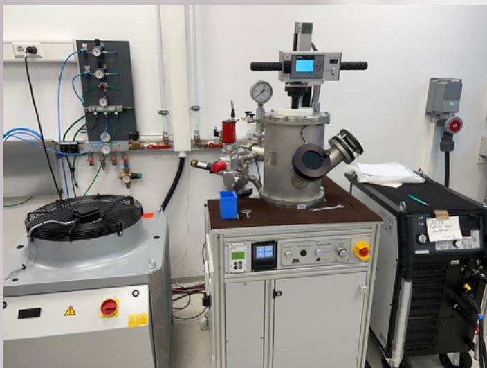
Figure: Arc melting device at NOMATEN. It will allow melting samples of up to approx. 200 g at temperatures up to 3500°C
